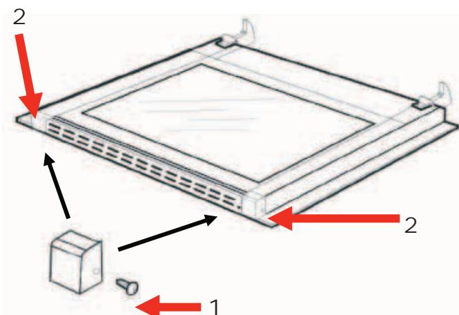
To remove the inner pane, screw out the screw 1 and open the plastic latches 2 located in the upper corners of the door. Now pull the glass carefully to set it free from the second blocking device. Take the glass out. Insert the clean glass back carefully and lock it by means of the blocking device.
