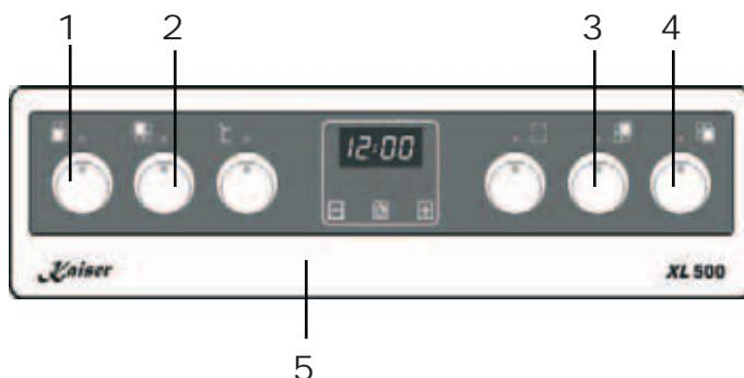
The cooking zones control is achieved by means of knobs 1, 2, 3 and 4 set up on the control panel of the cooker 5.
