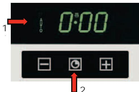
The symbols 1 ( AUTO ) and 0.00 start to flash if the device is switched on for the first time.
